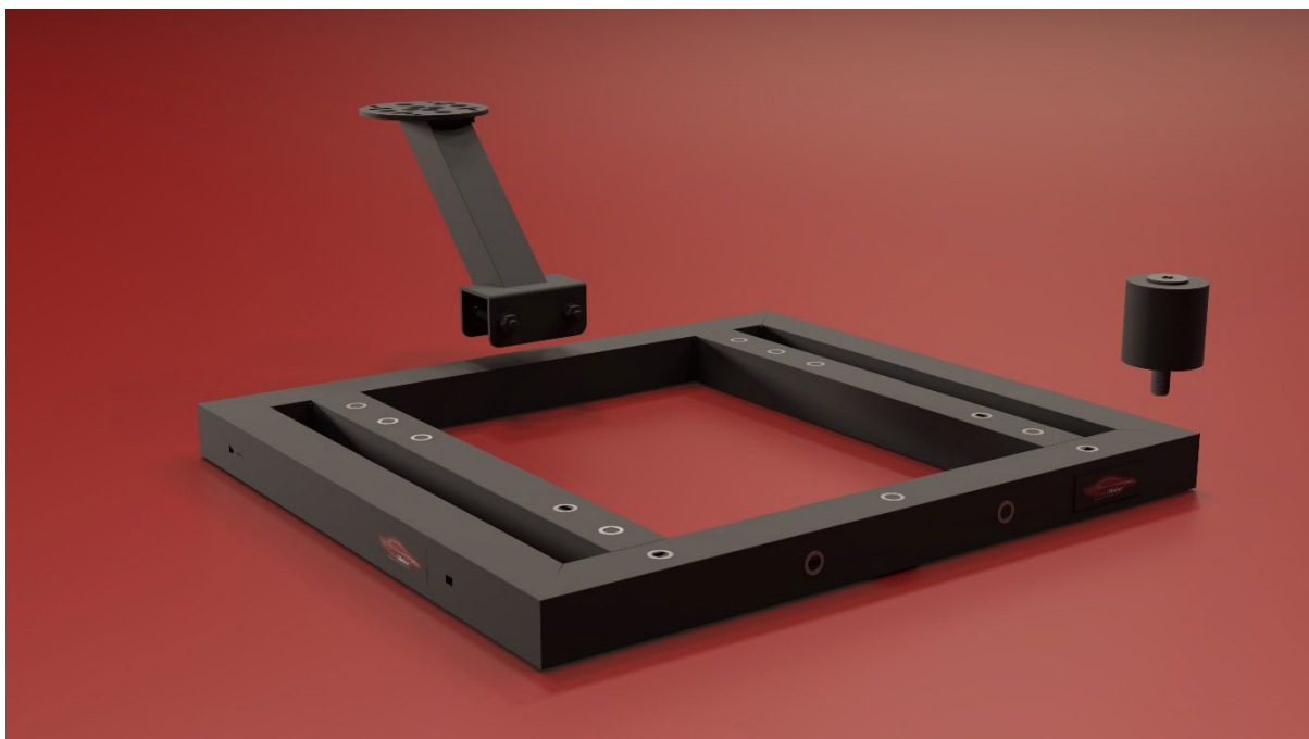
Figure 58: F2M seat frame exploded view
