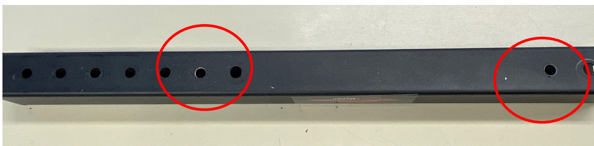
Figure 23: Additional drill holes
