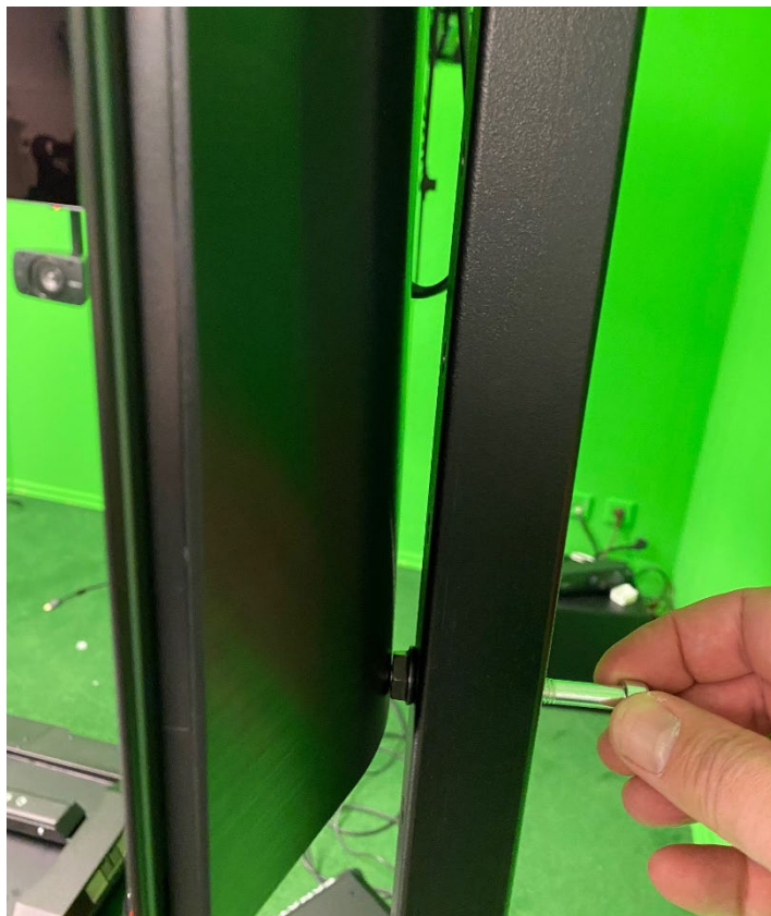
Figure 61 Tip: Support vertical mounting with set screw
